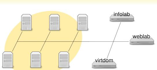
The prototype has been implemented on the University of Perugia Physics Department Computer Science Laboratory. The 35 diskless workstations were equipped with Xen 3.x using a shared NFS root filesystem hosted on the boot server virtdom.
