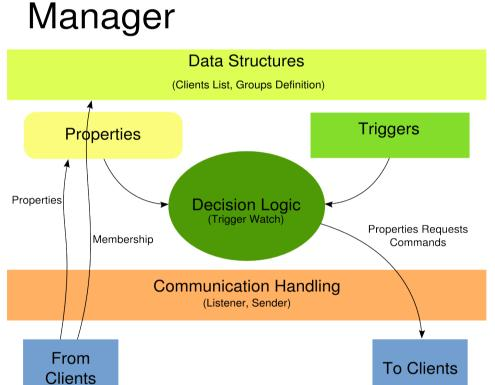
As well as the Client the Manager is written in python and consists of various threads: two for communication (Listener, Sender) and one for decision logic (TriggerWatch).
